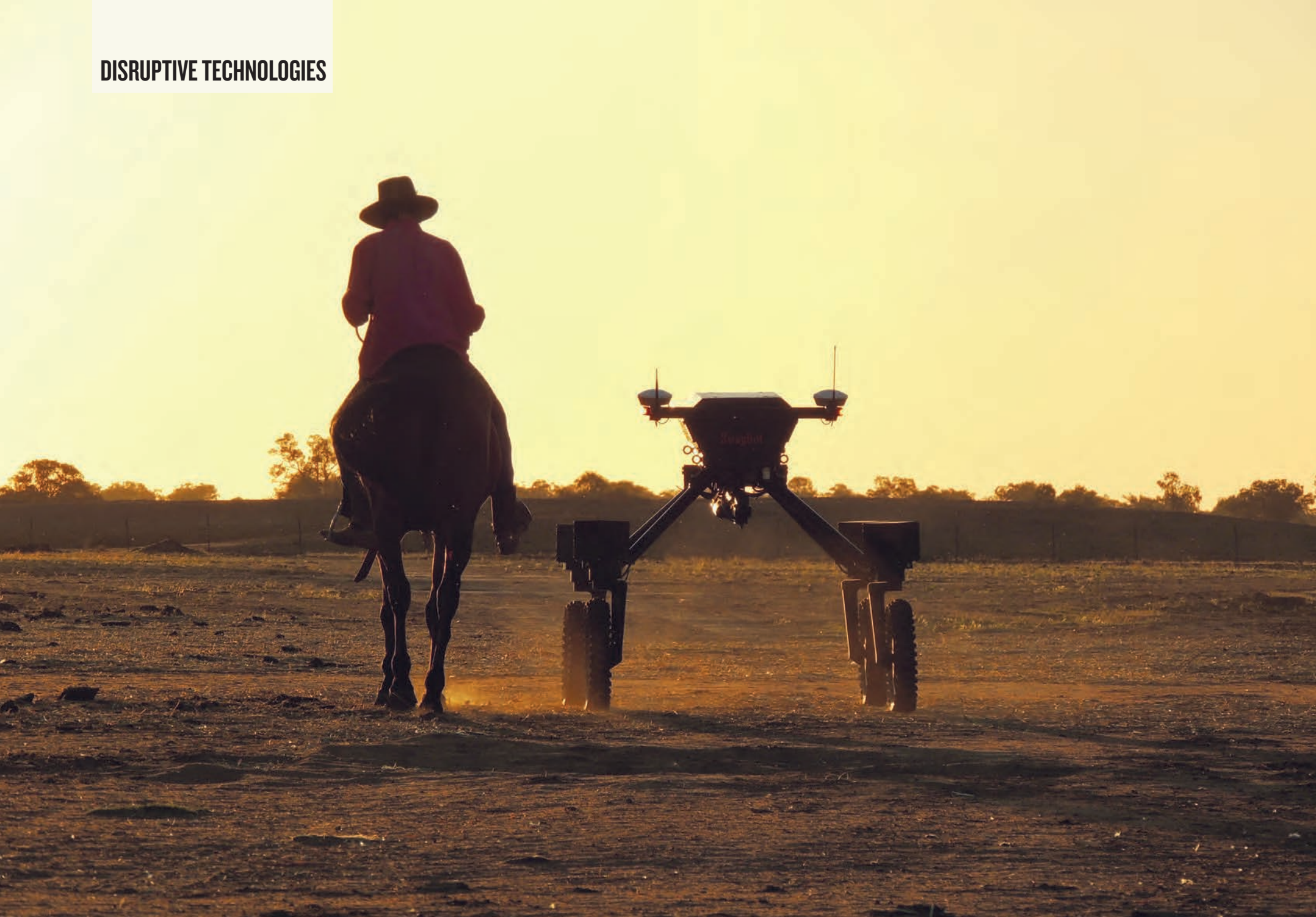
SwagBot, developed by the ACFR, is an autonomous vehicle designed for use on grazing livestock farms.
